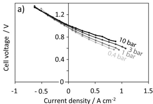
Figure 1. i-V curves measured on a 16 cm<sup>2</sup> planar SOC at 750°C. The i-V curves were obtained with 50% H<sub>2</sub>+50% H<sub>2</sub>O (24 l/h) supplied to the Ni/YSZ-electrode and 50 l/h O<sub>2</sub> supplied to the LSM/YSZ-electrode.
